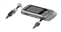
Warning!: Before connecting the Sway<sup>™</sup> to your PC with a USB cable, ensure your Sway<sup>™</sup> is not locked.
