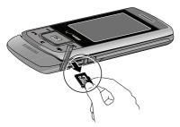
2. Press in the microSD card to unlock and remove.
