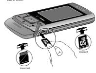
2. Push the microSD card into the slot until it locks into place.
